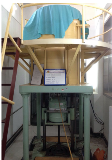
Figure 4.1 HPGe(THU) detector layout. Where the top of the detector consists of one shielding material (including lead, paraffin and SST) and PMT's. The bottom of the detector is filled with the N_2 gas to suppress the environmental backgrounds.
