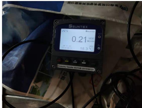
Figure 4.11 Panel of the water resistance sensor.
