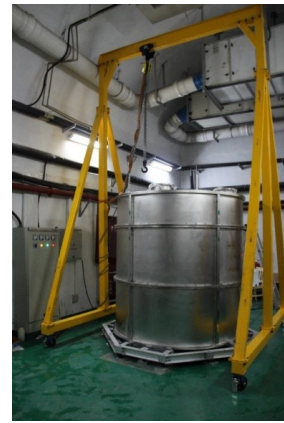
(d) Connect the middle and top parts of the tank with the bottom part.
