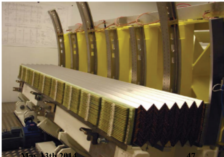
Fig. 2. One partly stacked module. The 6 outer rings on which are screwed the absorbers can be seen. Also the backbone (yellow part) and the assembling bench
