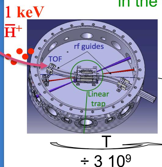
Capture and sympathetic Doppler cooling by laser cooled Be<sup>+</sup> ions in the linear **capture trap** (Paul trap,  $r_0 = 3.5$  mm,  $\Omega = 13$  MHz)
